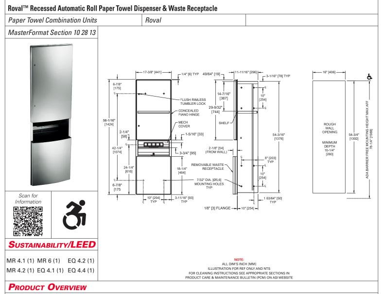
Proximity sensing no-touch unit dispenses a pre-set length per cycle from 8" [205] or 9" [230] wide standard towel roll up to 800 ft. (244m) long and has stub roll capability for continuous dispensing. Smaller waste receptacle, 13.5 gal. (51.1 L), allows unit to be ADA compliant. Internal shelf is ideal for paper towel storage. Towel length is determined by owner by setting length, delay and paper saver switches. Powered by 4 D-size batteries (not included).
