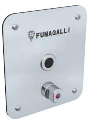
Recessed anti vandal shower mixer, ON/OFF working system. With optical sensor with settable parameters, filter, flow regulator and non-return valves. Conceived to reduce hand contact with the tap. Apart from the parameters functioning setting, the exclusive DCS systems allows the recording and the visualization of the historical data.
