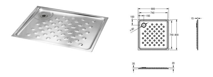
Shower tray for recessed mounting, stainless steel, surface satin finished, material thickness 1 mm, deepdrawn out of one piece with rounded internal corners, bowl slanted towards waste, slip resistant patterned foot areas, waste  $\emptyset$  90 mm, corners welded, earthing lug welded at bottom, no waste included.
