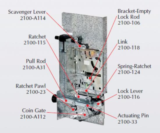
Rear View of Coin Mechanism
